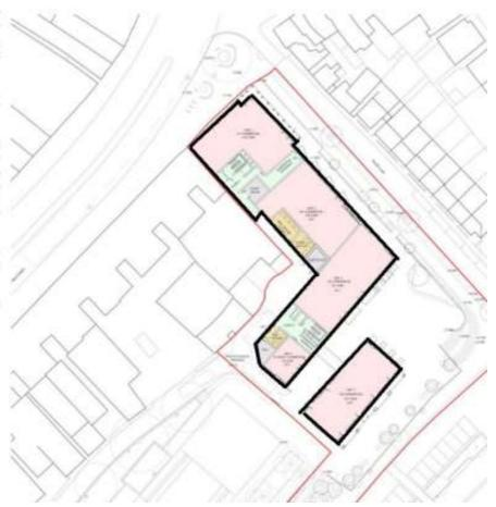
Image: Proposed Ground Floor Plan (planning application: design and access statement). The planned building footprint is outlined in black for clarity. The planning site boundary, which includes pavements and some street parking spaces is outlined in red.
